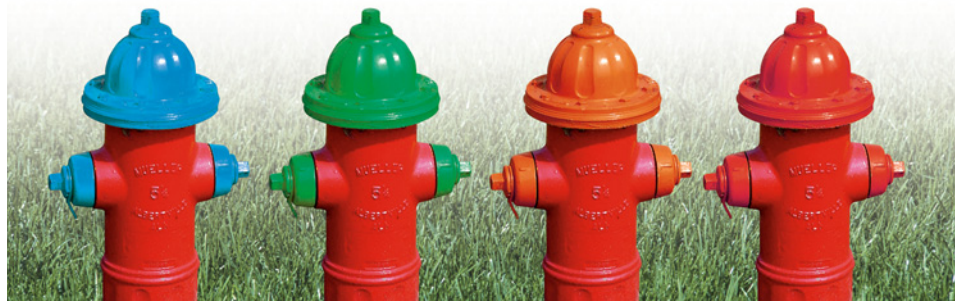
Go with the flow. Hydrants in the township are being repainted to signal their flow rates. Red is under 500 gallons per minute; Orange is 500 to 999; Green is 1,000 to 1,500; blue is over 1,500.
