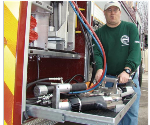
Power tools. Rescue Officer Steve Dancisin explains the operation of the cutting and spreading tools carried on the Fire Company's rescue truck used to extricate trapped passengers. Dancisin was part of a committee that specified every detail of the new rescue truck, which was delivered last year. ~
