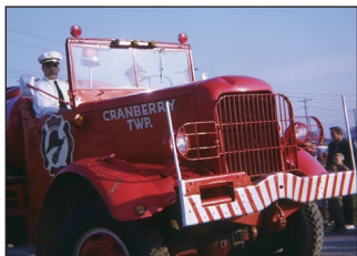
This tanker built onto a military truck chassis was part of the Fire Company’s early fleet.
