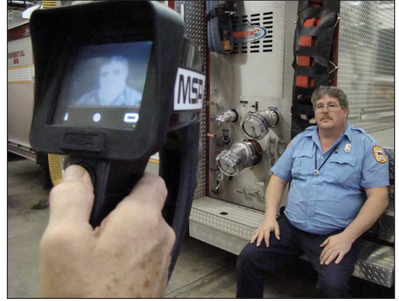
Gottcha. The picture of Fire Company Administrative Assistant Mark Nanna captured on the display of this MSA thermal imaging camera was created from infrared radiation rather than visible light. The rugged cameras, which are carried on every CTVFC fire truck, can see heat sources, including concealed fires, right through a building's walls and ceilings.
