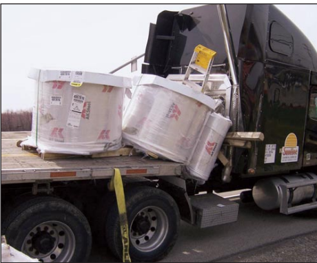
The truck stops here. Cranberry police cited the driver of this rig on Rt. 228 after its load of steel coils, illegally secured with canvas straps alone, shifted and rolled onto the highway as well as into his cab. Township police have stepped up their truck safety inspections over the past two years.
