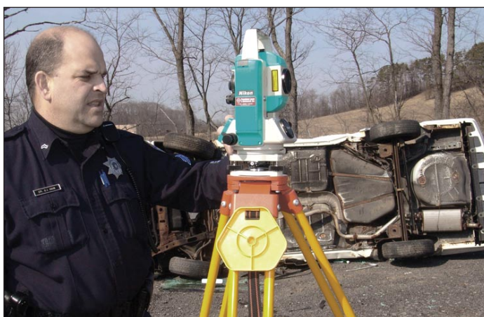
Off road vehicle. Cranberry police Cpl. Daniel Hahn uses an instrument similar to a surveyor's transit to establish vehicle speeds and trajectories in reconstructing how traffic accidents occurred.
