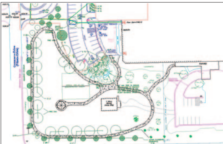
Down the trail. This engineering schematic shows the alignment of a 1/5-mile walking trail as well as the placement of shade trees and a new gazebo, which will be installed this spring at the northeast corner of Cranberry Township's Municipal Center property on Rochester Road.
