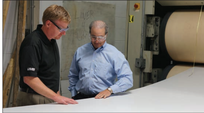
Check it out. US Liner V.P. of Sales and Marketing Jeff Meek, left, and company CEO Michael LaRocco, inspect composite sheet coming off the lamination press in the firm's Cranberry plant. Variations of the rugged material are used to protect interior compartments on refrigerated trailers and shipping containers worldwide.
